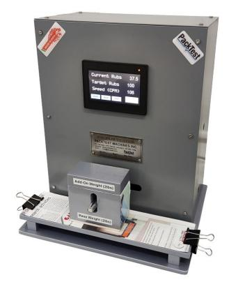
**Model # QXT** Touchscreen model with 4 Speeds of rubbing (selectable): 21, 42, 85 and 106 CPM Supplied with 2 Lbs and 4 Lbs (2 + 2 addon) rubbing weights to vary the rubbing pressure.
