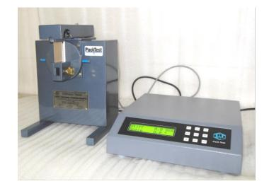
Automatic Test Cycle. (Upon pressing Start, the Stiffness Tester will record the 15° Stiffness on Left Side and then 15° Stiffness on Right Side and come back to center parking position).
