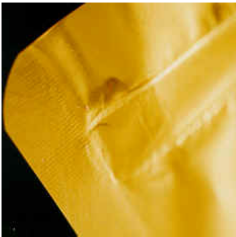
No cross-over sealing of the primary seal with the side seal
