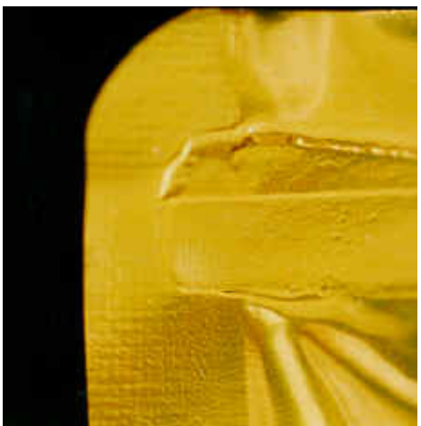
No cross-over sealing of the primary seal with the side seal
