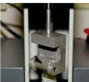
Figure 4.6 Tensile Test Equipment Showing a Sample Being Tested Sample Test Strip Positioned in Clamps
